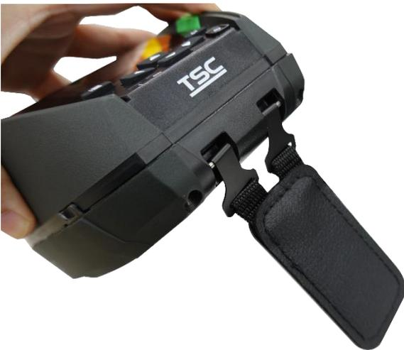
9. Press the hook of belt clip into the bars on the lower printer as pictured. The printer can be hung on the belt.
