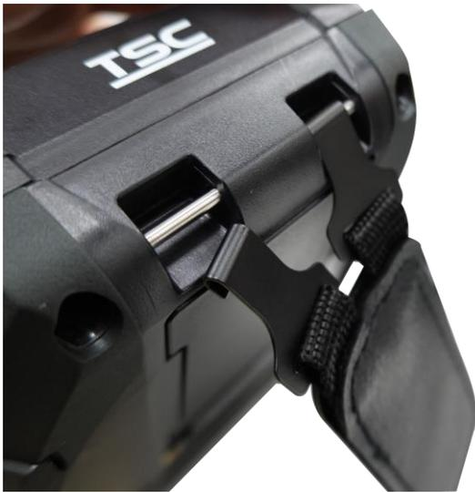
8. Lock the belt clip on lower of the printer.
