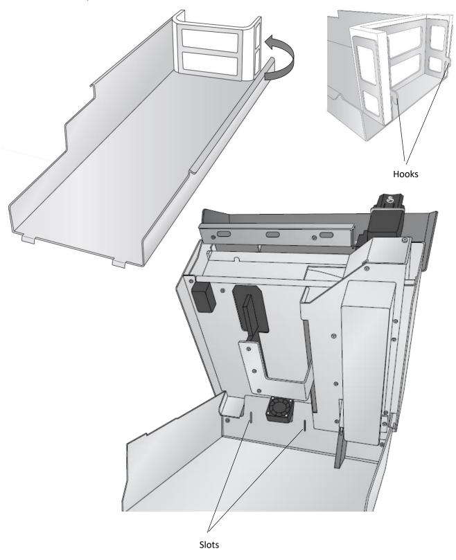
• Install the Crumb Catcher by inserting the hooks into the slots. You will see the hooks through the slots on the back of the printer. Align the front Crumb Catcher tabs on either side of the Carousel Base connection bracket.
