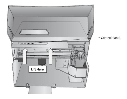
• The top section of the printer will open and stay open with a gas spring. As long as the power is on, the print item platform will move up and out of the way so you may install the Crumb Catcher.
