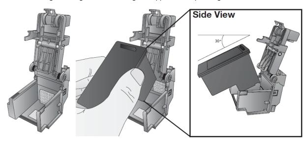
6. Make sure the cartridge is pushed back far enough so the ridge on the cartridge is behind the spring-loaded pusher on the lid. <u>Push down on the cartridge</u>. Close the lid on the cartridge by lightly pressing down from the top until you hear a click.
