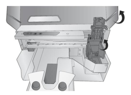
2. Press or pinch the tab on the front of the cartridge holder.
