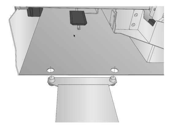
• Locate the 6 Pin Mini Din Cable attached to the Carousel Base. Route the cable along the left side of the unit until it reaches the back of the printer. Open the Top Cover.
