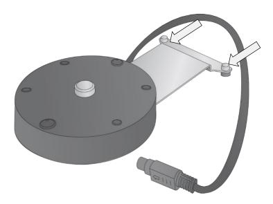
• Lift the base of the printer slightly and slide the carousel base underneath. Align the holes with the pins and lower the printer into place.
