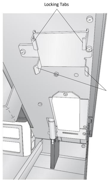
**Note:** To remove or insert the ink trough squeeze the ink trough not the tabs.
