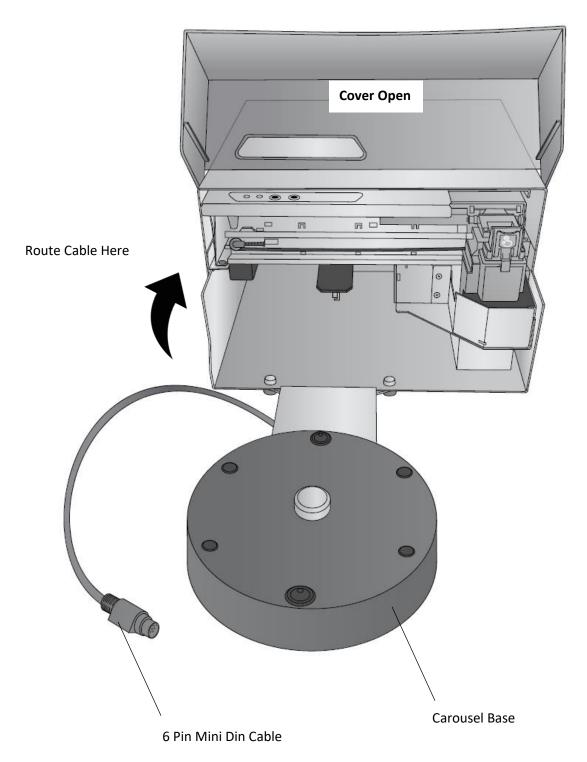
• Connect the 6 Pin Mini Din Cable to the round port on the back of the printer.
