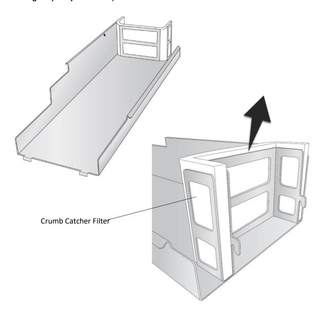
To remove the Crumb Catcher from the printer first remove the Carousel Tray and then lift up on the top section of the printer. Power should be connected at this point, so the Print Item Platform is moved out of the way. Now you may access the Crumb Catcher. Lift near the back to disengage the hooks that secure it to the back of the printer.
