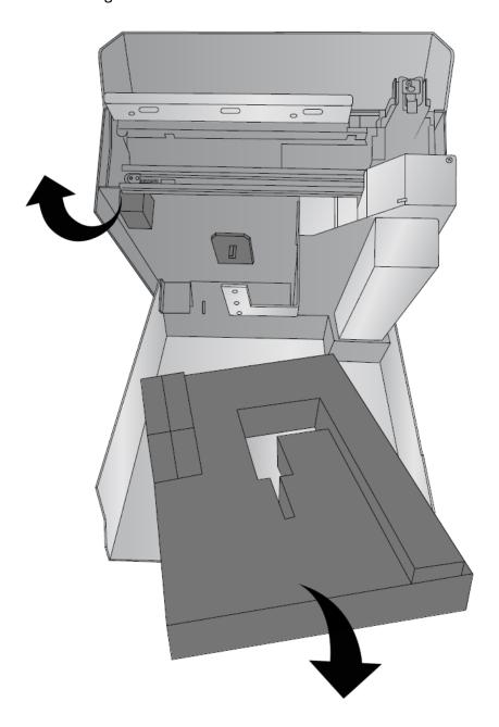
Locate the Carousel positioning holes in the base.
