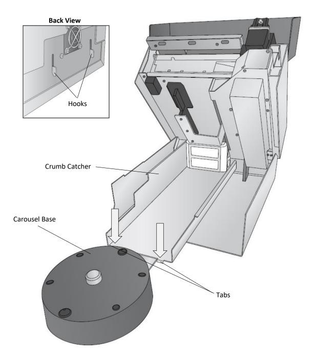
• Lower the Top Section of the Printer.
