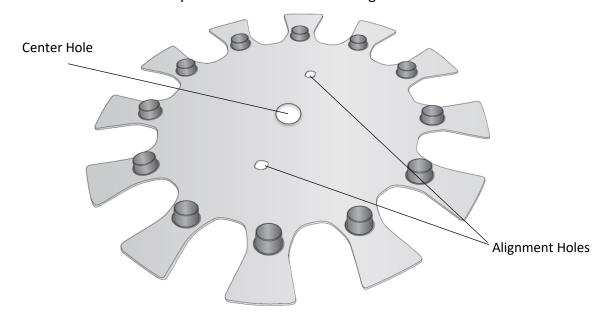
• Install the tray by aligning the center hole with Center Hub on the Carousel Tray base. Rotate the tray by hand until the holes in the tray are aligned with the pegs on the base.
