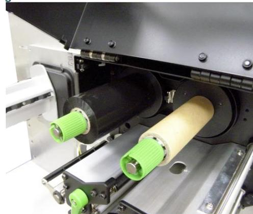
3. Push print head release lever to open print head mechanism.
