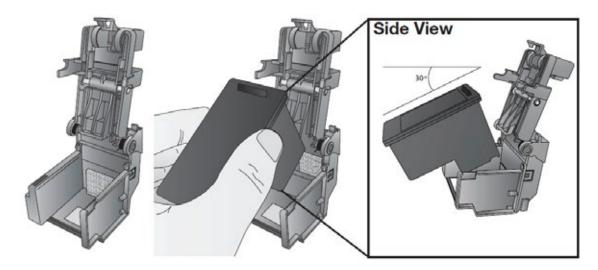
6. Make sure the cartridge is pushed back far enough so the ridge on the cartridge is behind the spring-loaded pusher on the lid. <u>Push down on the cartridge</u>. Close the lid on the cartridge by lightly pressing down from the top until you hear a click.
