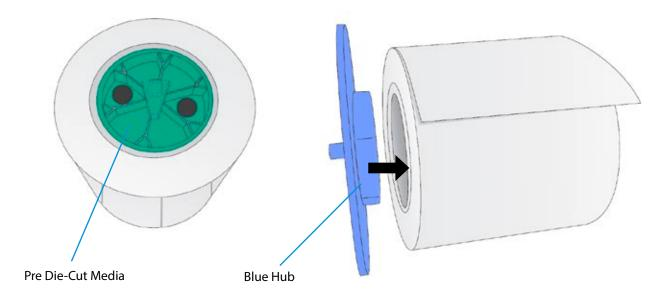
4. Set the roll in place so that the blue pin sits in the notch on the roll holder.
