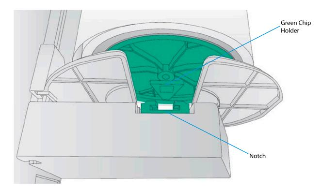
5. Make sure the green blank chip holder fits in the corresponding green slot on the roll holder.
