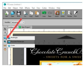
2. Before you start to draw the cut line, adjust the corner radius. You will not be able to change this after you draw your cut line. The corner radius is the amount of curve around the corners. .125 in (1/8 Inch) is the standard corner radius.
