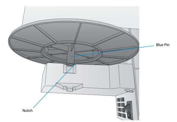
3. Set the roll in place so that the blue pin sits in the notch on the roll holder.
