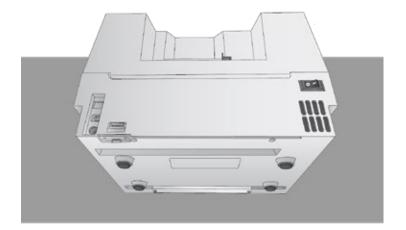
2. Install the movable label roll holder by attaching the hooked end on the rail. The bottom of the holder will fit in the notch on the printer.
