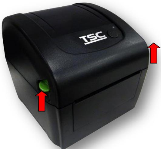
A black TSC printer is shown from a three-quarter perspective. Two red arrows point upwards to the top latches on the left and right sides of the printer's lid, indicating where to press to open it.                                          | <ol style="list-style-type: none"><li>1. Aprire il coperchio della stampante premendo le linguette d'apertura copertura superiore su ciascun lato della stampante.</li></ol> |
