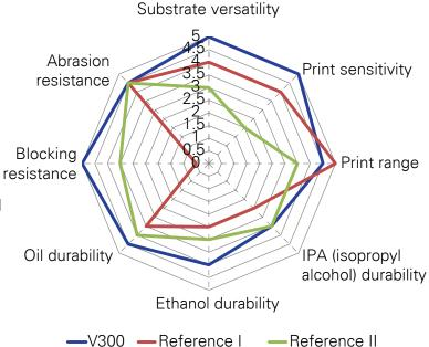
The graph showcases an average of results based on tests printed with Zebra 140xi4, SATO408Rex, on PET, PP and paper
