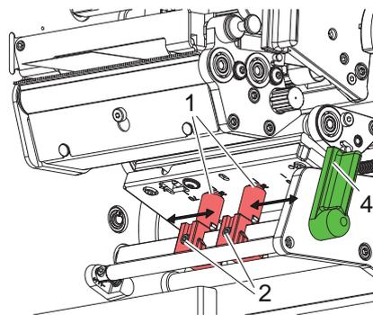
Figure 17 Setting the lower head locking system
