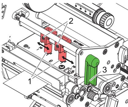
Figure 16 Setting the upper head locking system
