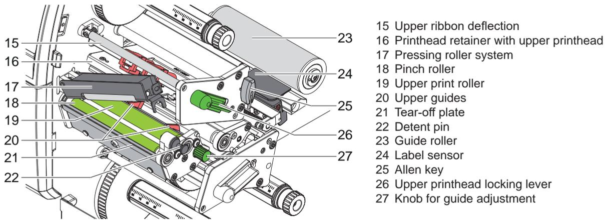
Figure 3 Print mechanics - upper print unit
