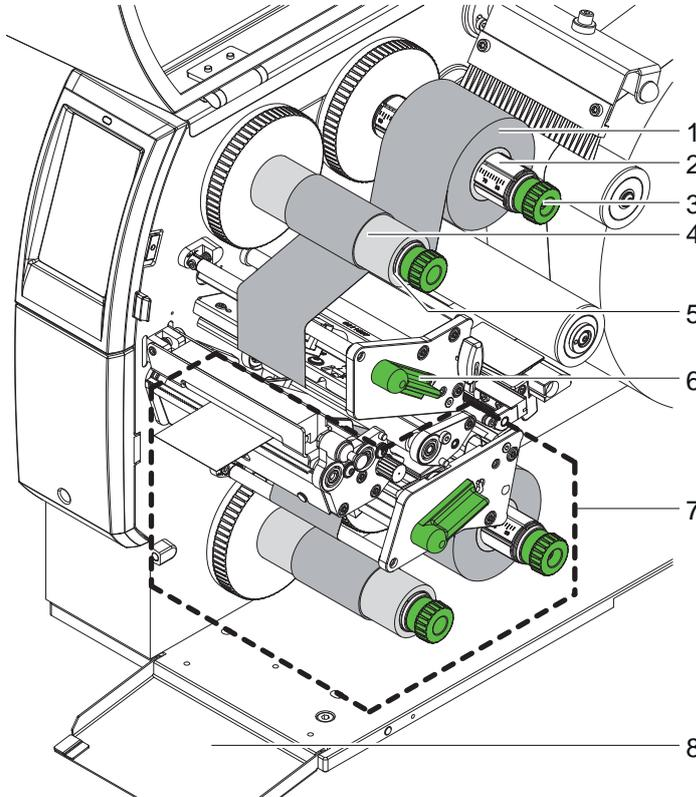
Figure 18 Load transfer ribbon
