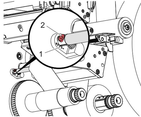
Figure 21 Setting the lower ribbon feed path
