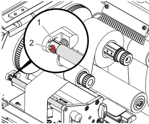
Figure 20 Setting the upper ribbon feed path
