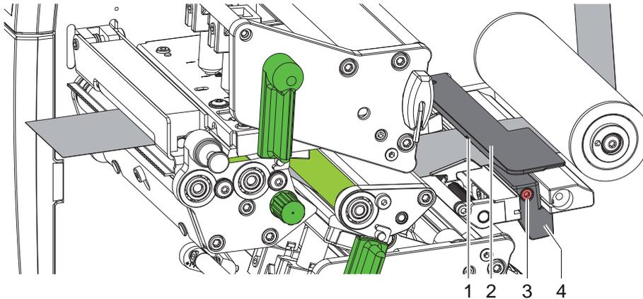
Figure 15 Setting the label sensor
