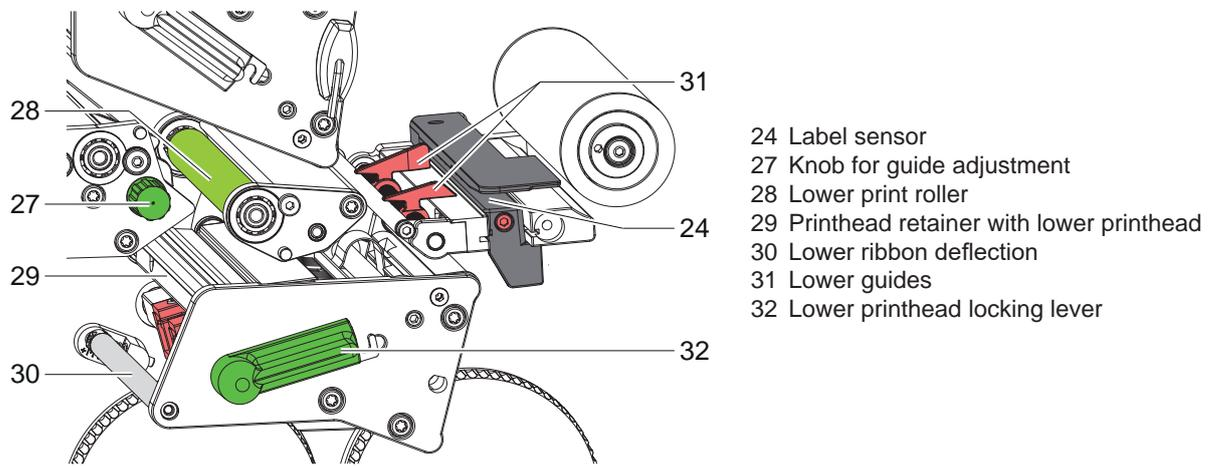
Figure 4 Print mechanics - lower print unit
